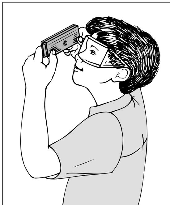
**Figure 3-1.** Using a Pocketscope to view a powder.
