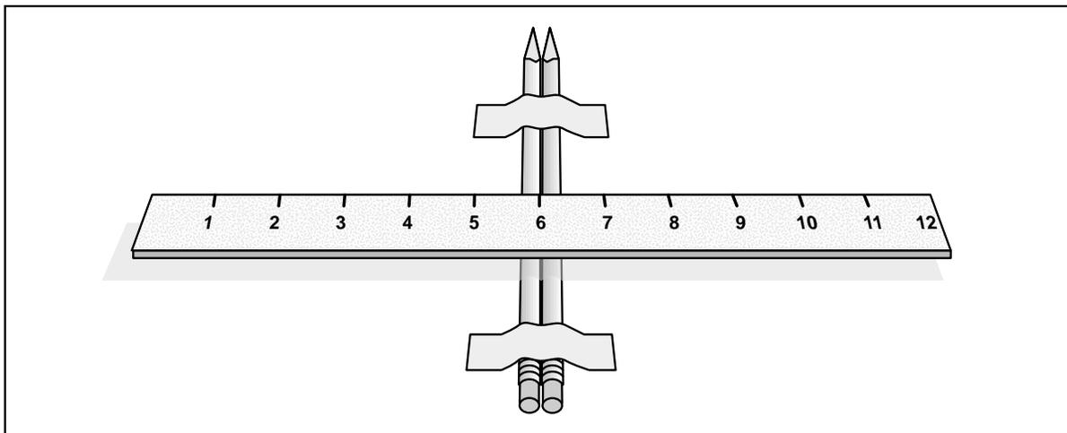
Figure 2-2. Making a lever from a ruler and two pencils.
