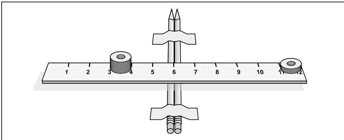
Figure 2-3. Moving the load closer to the fulcrum reduces the length of the load arm as well as the effort needed to lift the load.
