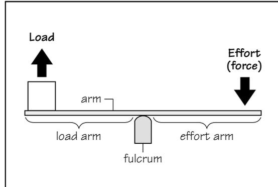
Figure 2-1. The parts of a lever.
