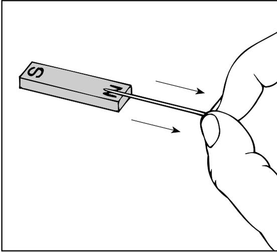
Figure 5-1. Magnetize the needle by stroking it against the north pole of a bar magnet.
