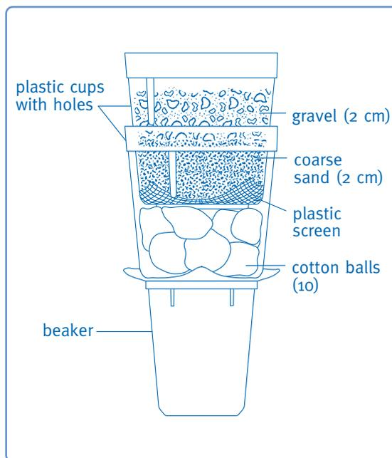
▲ Figure 5-2. The completed water filtration system.
